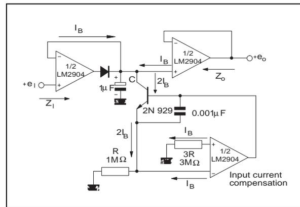
USING SYMMETRICAL AMPLIFIERS TO REDUCE INPUT CURRENT
