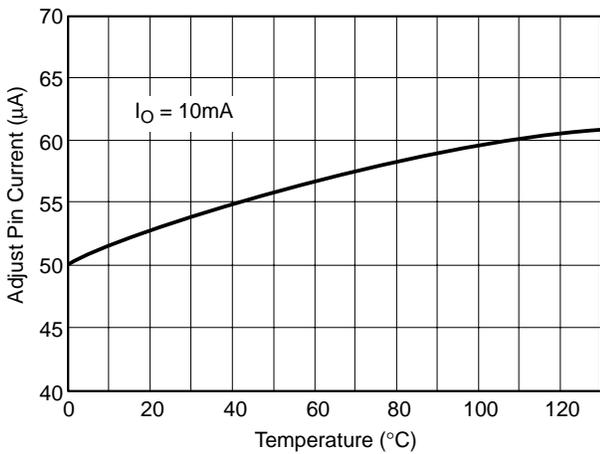
Figure 7. Adjust Pin Current vs. Temperature (Adjustable Output)
