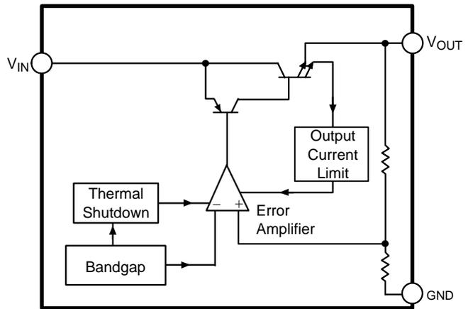
Figure 4. Block Diagram, 3.3 V Fixed Output
