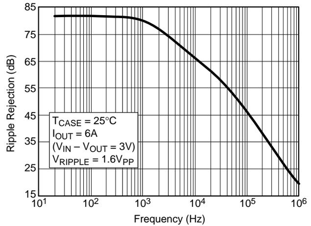
Figure 12. Ripple Rejection vs. Frequency (3.3 V Fixed Output)
