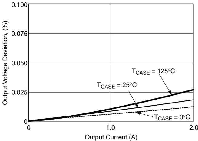
Figure 13. Load Regulation vs. Output Current (Adjustable Output)
