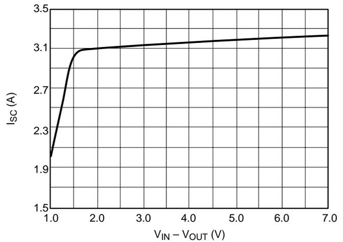
Figure 8. Short Circuit Current vs.  $V_{IN} - V_{OUT}$
