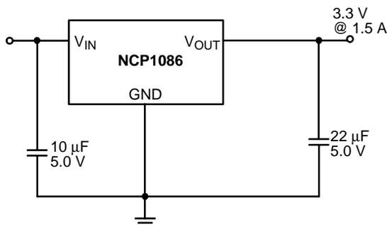
Figure 2. Application Diagram, 3.3 V Fixed Output
