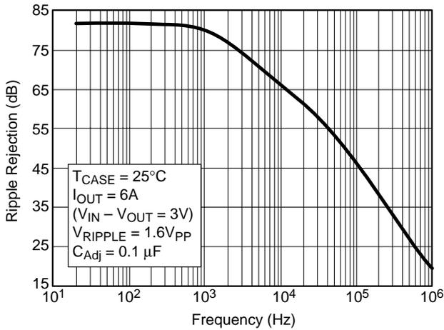
Figure 11. Ripple Rejection vs. Frequency (Adjustable Output)
