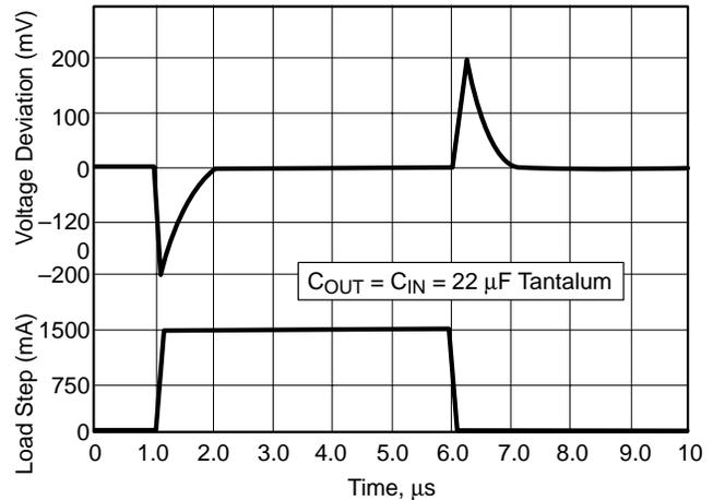
Figure 10. Transient Response (3.3 V Fixed Output)
