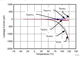
Figure 37. Leakage Current vs Temperature
