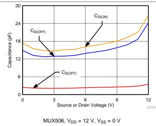
Figure 23. Capacitance vs Source Voltage
