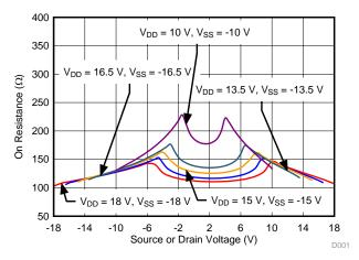
Figure 41. On-resistance vs Source or Drain Voltage
