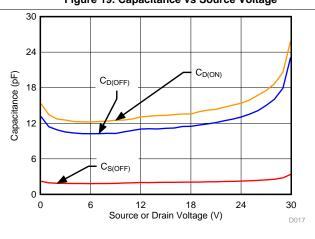
MUX506,  $V_{DD} = 30 \text{ V}$ ,  $V_{SS} = 0 \text{ V}$
