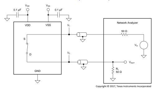
Figure 35. Bandwidth Measurement Setup
