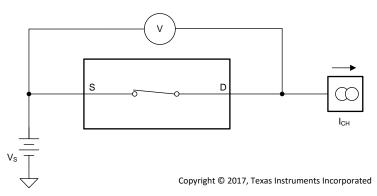
Figure 26. On-Resistance Measurement Setup
