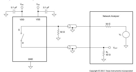
Figure 33. Off Isolation Measurement Setup
