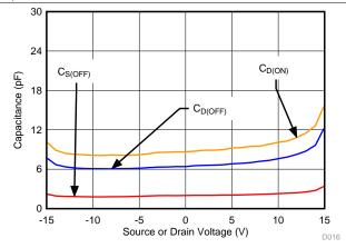
MUX507,  $V_{DD} = 15 \text{ V}$ ,  $V_{SS} = -15 \text{ V}$
