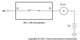
Figure 28. On-Leakage Measurement Setup
