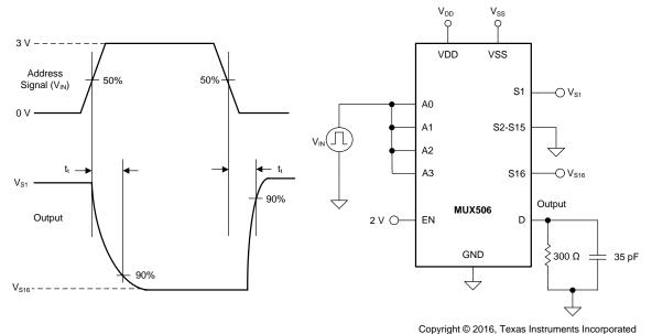
Figure 29. Transition-Time Measurement Setup
