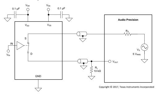
Figure 36. THD+N Measurement Setup
