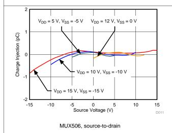
Figure 11. Charge Injection vs Source Voltage
