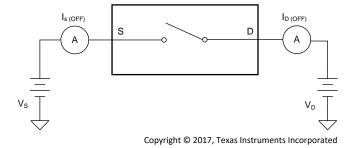
Figure 27. Off-Leakage Measurement Setup
