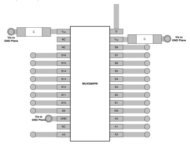
Figure 45. MUX506IPW Layout Example
