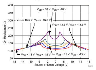
Figure 44. On-Resistance Variation With Supply and Input Voltage
