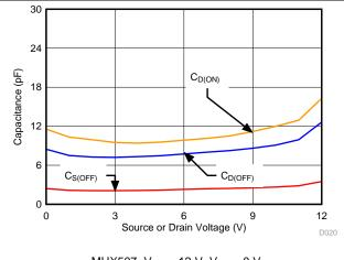
MUX507,  $V_{DD} = 12 \text{ V}$ ,  $V_{SS} = 0 \text{ V}$
