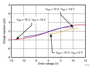
Figure 40. Drain-to-Source Charge Injection
