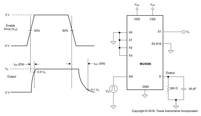
Figure 31. Turn-On and Turn-Off Time Measurement Setup
