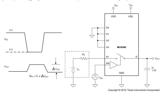
Figure 32. Charge-Injection Measurement Setup
