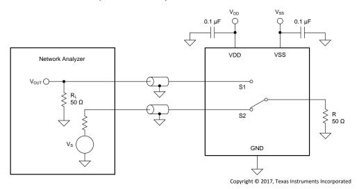
Figure 34. Channel-to-Channel Crosstalk Measurement Setup
