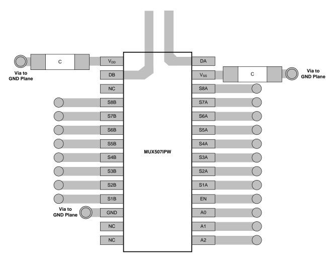
Figure 46. MUX507IPW Layout Example
