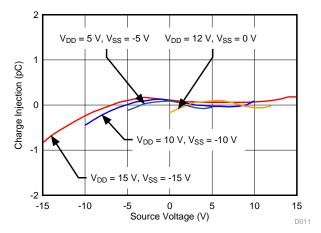
Figure 39. Source-to-Drain Charge Injection
