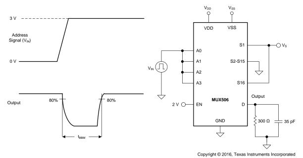
Figure 30. Break-Before-Make Delay Measurement Setup
