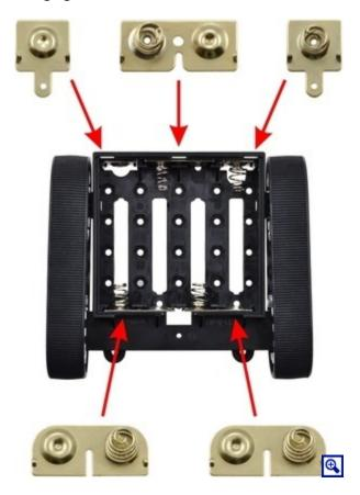
12. Insert four AA batteries (the cut-out slots in the battery holder indicate the proper battery orientation) and snap the battery cover onto the bottom of the chassis.
