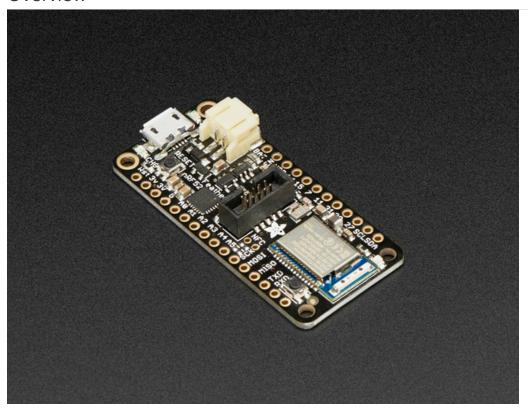
The Adafruit Feather nRF52 Pro is our latest Bluetooth Low Energy board for advanced projects and users who want to use a fully open source Bluetooth Low Energy 5.0 stack. It has a native-bluetooth chip, the nRF52832, as well as built in USB Serial and battery charging! We have other boards in the Feather family, check'em out here.
