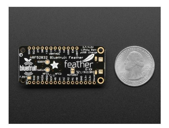
The Adafruit Feather nRF52 Pro ships pre-programmed with the Mynewt serial bootloader that allows you to flash firmware to the device directly from the command-line using the on-board USB Serial converter and the 'newtmgr' tool, so you can get started right away with no additional hardware required. For more advanced debugging, however, you can use a Segger J-Link and the on-board SWD debug connector, which gives you access to a more powerful set of development tools and options.
