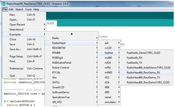
Before uploading, check for the #define FREQUENCY RF69\_915MHZ line and comment that out (and uncomment the line above) to match the frequency of the hardware you're using
