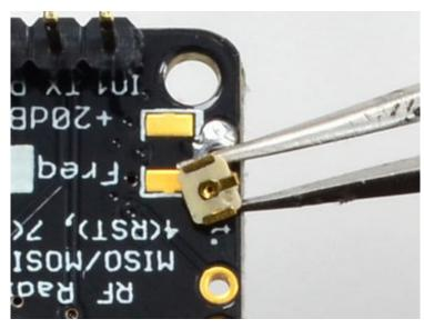
Check the bottom of the uFL connector, note that there's two large side pads (ground) and a little inlet pad. The other small pad is not used!
