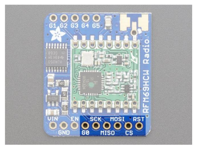
All pins going into the breakout have level shifting circuitry to make them 3-5V logic level safe. Use whatever logic level is on **Vin!**
