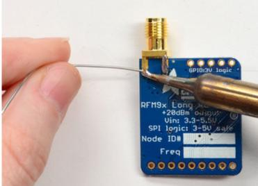
Flip over and also do the other side ground/mechanical contacts
