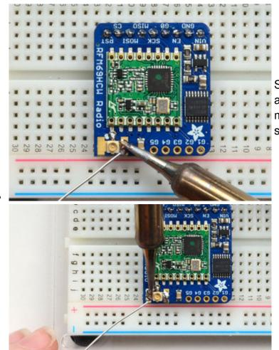
Solder in the two side pads, they are used for signal and mechanical connectivity so make sure there's plenty of solder
