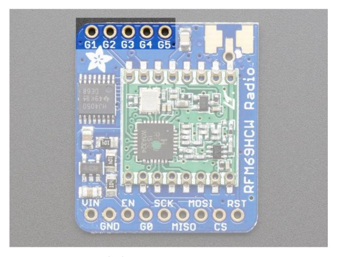
The radio's have another 5 GPIO pins that can be used for various notifications or radio functions. These aren't used for the majority of uses but are available in case you want them! All are 3.3V logic with no level shifting
