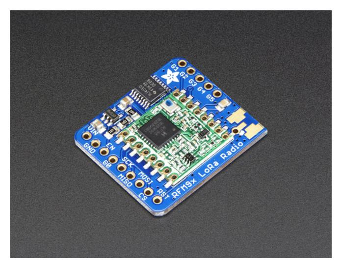
Note that the sub-GHz radio is not designed for streaming audio or video! It's best used for small packets of data. The data rate is adjustbale but its common to stick to around 19.2 Kbps (thats bits per second). Lower data rates will be more successful in their transmissions
