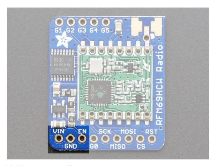
The left-most pins are used for power
