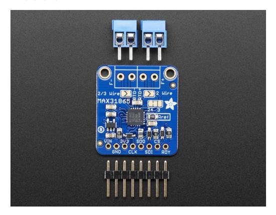
Each order comes with one assembled RTD amplifier breakout board. Also comes with two 2-pin terminal blocks (for connecting to the RTD sensor) and pin header (to plug into any breadboard or perfboard). A required PT100 or PT1000 RTD is not included! (But we stock them in the shop). Some soldering is required to solder the headers and terminal blocks to the breakout, but it's an easy task with soldering tools.
