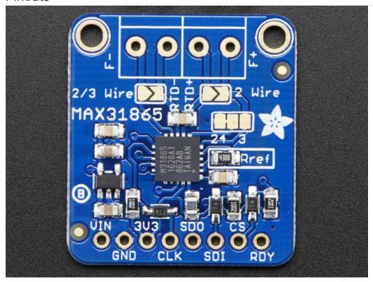
The MAX31865 is a tiny surface mount chip, and it needs a lot of other parts to make it work, so we've got it on a nice breakout board for you. You can control the chip and read data from it using the breakouts at the bottom. Let's go thru these!
