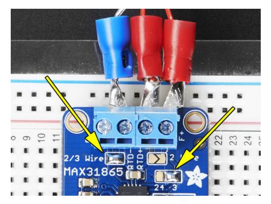
You will have to cut the thin trace in between the 2-way jumper on the right side of the board, and then solder closed the blob on the right side.
